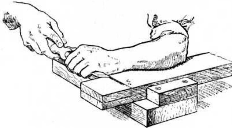
**Fig. 66.—Chiselling away Wood up to Gauge Line.**
