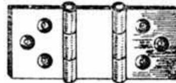
Fig. 232.—Non-reversible Screen Hinge.
