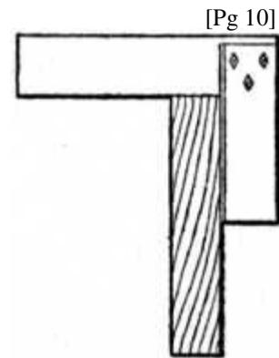
Fig. 22.—Use of the Try-square for Testing Edge.
