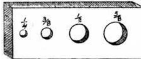
**Fig. 190.—Steel Dowel Plate.**
