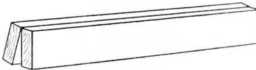
**Fig. 2.—How the Wood is held whilst Glueing.**
