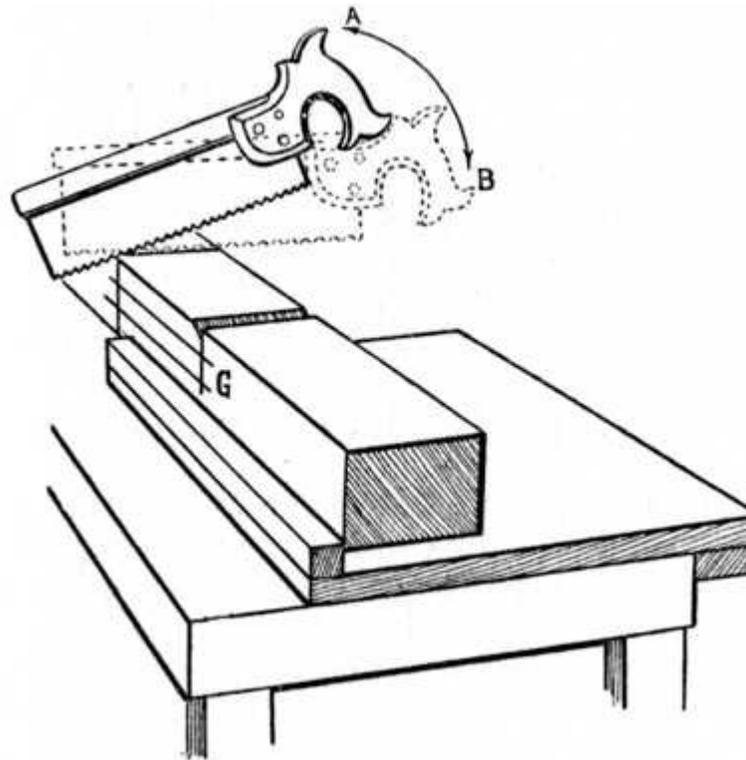
**Fig. 89.—Sawing the Shoulders.**
