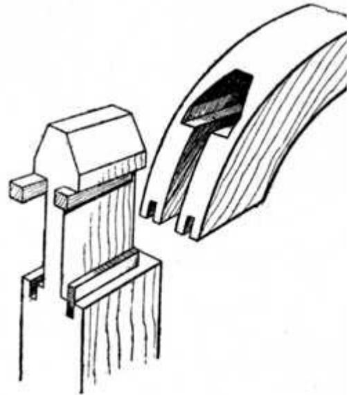
**Fig. 171.**—Hammer-Head Tenon Joint
