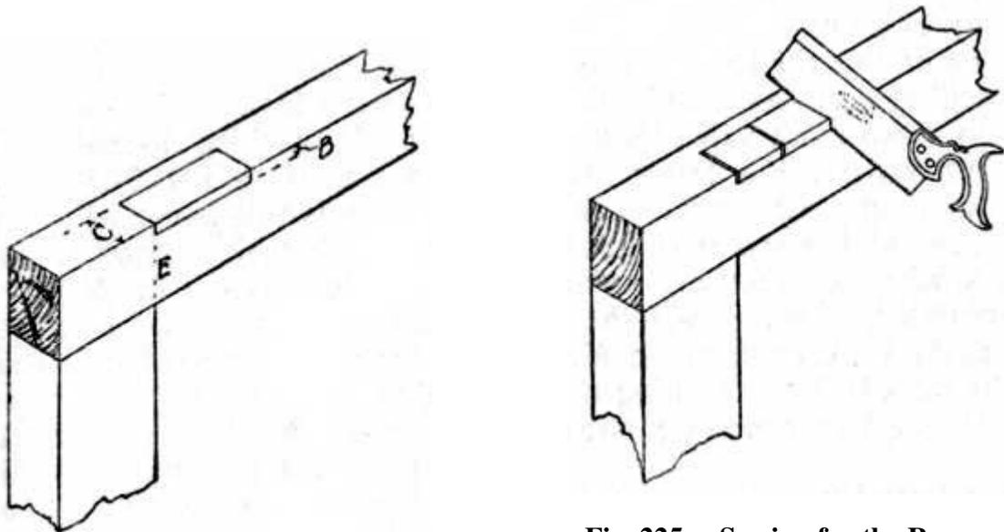
Fig. 225.—Sawing for the Recess.
