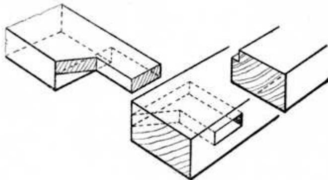
**Fig. 142.—Haunched Tenon for Skylight or Garden Frame.**
