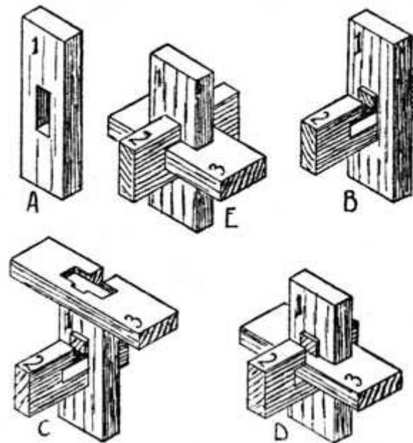
**Fig. 389.—Mortising Puzzle, showing how the Parts Fit.**
