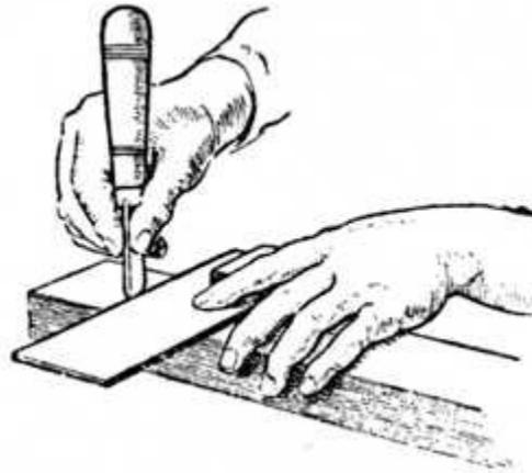
**Fig. 64.—Marking the Joint with Try Square.**
