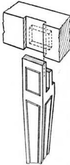
**Fig. 141.—Method of Fitting an Interior Table Leg.**
