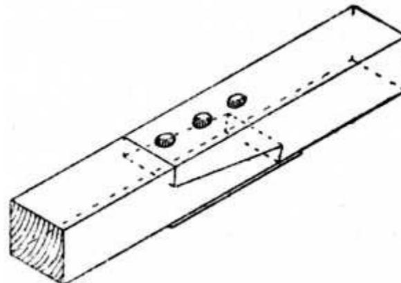
**Fig. 213.—Plated Scarf Joint Used in Roof Work.**
