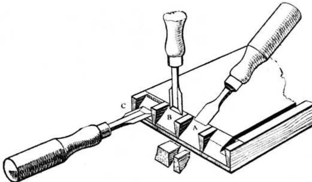
**Fig. 276.—Showing the Vertical and Horizontal Chisel Operations in Lap-dovetailing. A: The Preliminary Roughing-out. B: Vertical Chiselling; note that the first stab should be just outside the Gauge Line. C: Marking the Horizontal Cut.**
