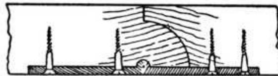
**Fig. 250.—Rule Joint Hinge, with Leaf Open.**
