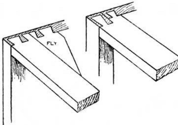
**Fig. 293.—Carcass Work, showing Bearer Rails
