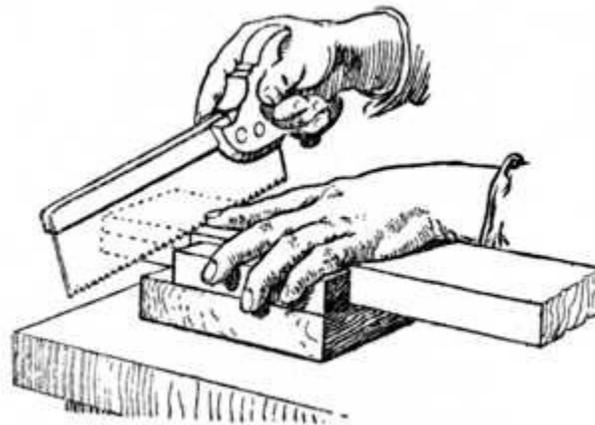
**Fig. 67.—How work is held when Sawing Shoulder.**
