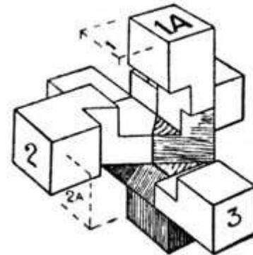
**Fig. 393.—Method of Putting Together.**
