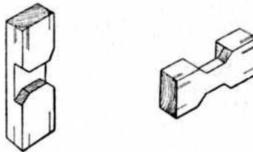
**Figs. 49 and 50.—Separate pieces of Halved Moulded Joint.**
