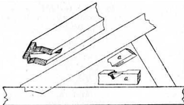
**Fig. 80.—Application of Bridle Joint to Roof Truss.**
