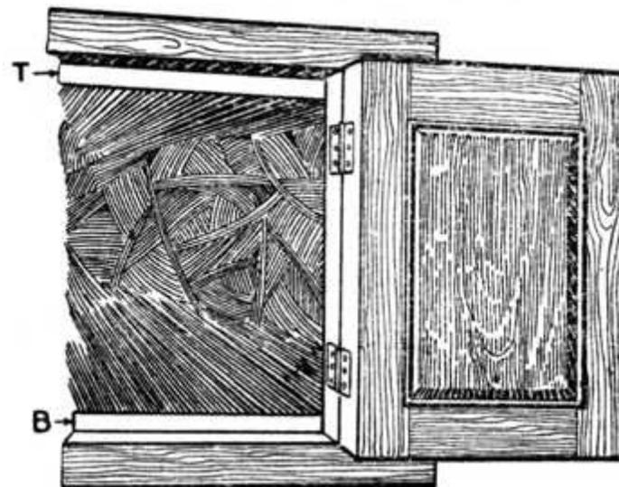
Fig. 239.—Showing Top and Bottom of Carcase Cut
