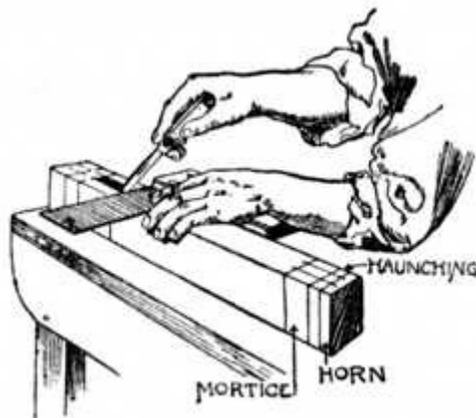
**Fig. 178.—Setting Out the Stiles with Marking Knife.**
