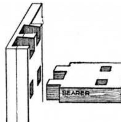
**Fig. 148.—Mitred and Moulded Tenon Joint.****Fig. 149.—Twin Tenons.**
