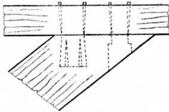
Fig. 174.—Inserted Tenons.
