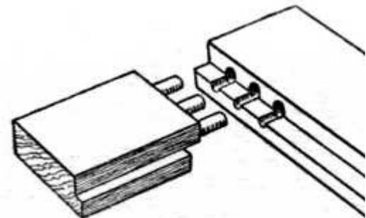
**Fig. 203.—Method of Frame Dowelling Short Shoulders.)**
