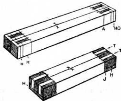
Fig. 177.—Setting out Stiles and Rails for Tenoning.
