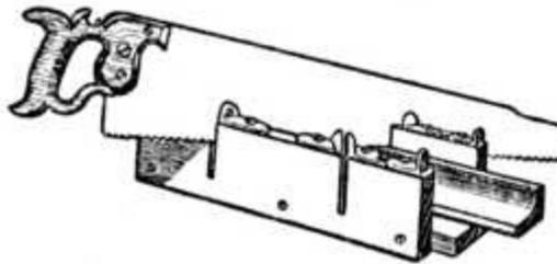
**Fig. 334.—Using Panel Saw in Mitre Box.**
