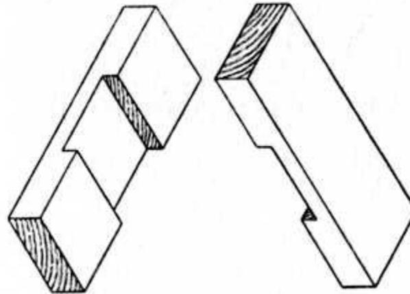
**Fig. 62.—The Two Pieces of a Halved Joint.**
