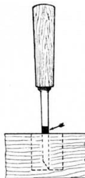
**Fig. 129.—Method of Gauging for depth of Tenon.**
