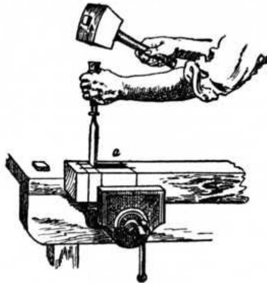
**Fig. 183.—Using the Chisel and Mallet
