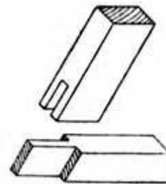
**Fig. 79.—Oblique Angle Bridle Joint**
