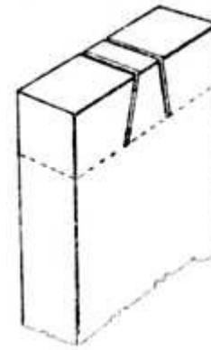
Fig. 280.—Gauge Lines, Scores and Sa Cuts.
