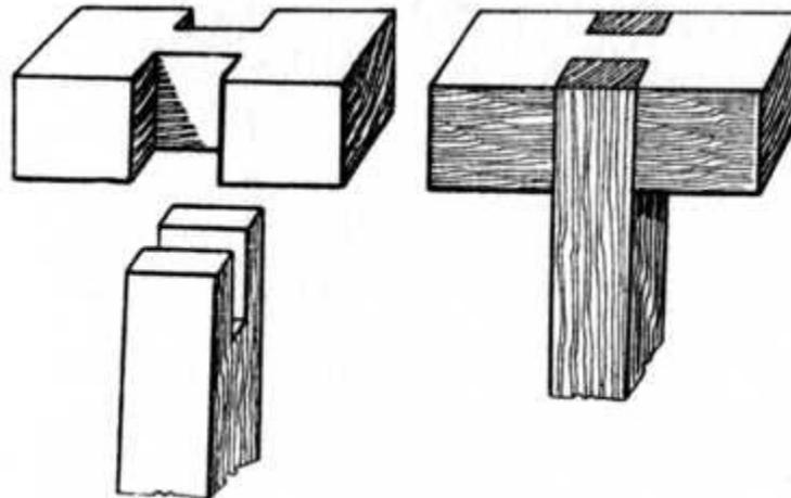
**Fig. 72.—Simple Bridle Joint.**
