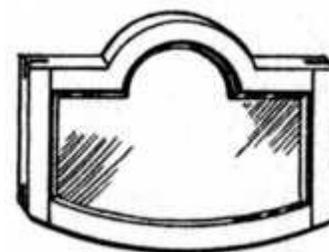
**Fig. 75.—Mirror Frame with Bridle Joints.**
