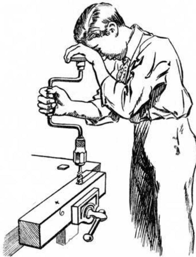
**Fig. 85.—Vertical Boring previous to Chiselling.**
