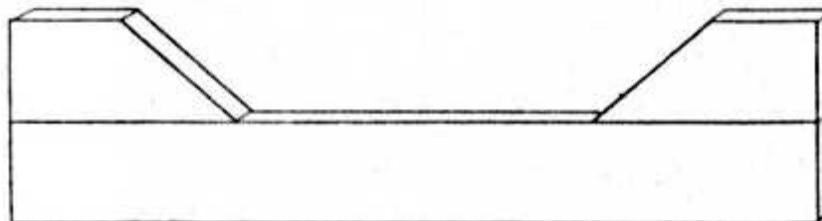
**Fig. 14.—Carcase Wing-pieces Glued on.**
