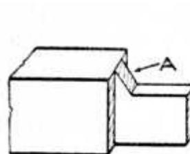
**Fig. 130.—Haunched Tenon used at end of Door Frame.**
