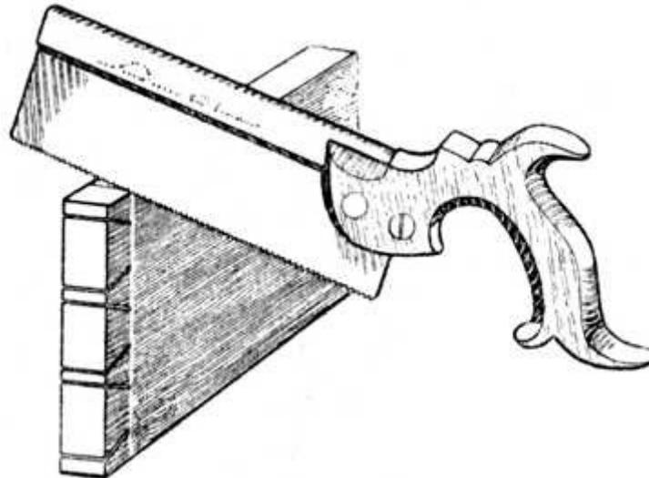
**Fig. 275.**—Cutting away the Half Dovetails.
