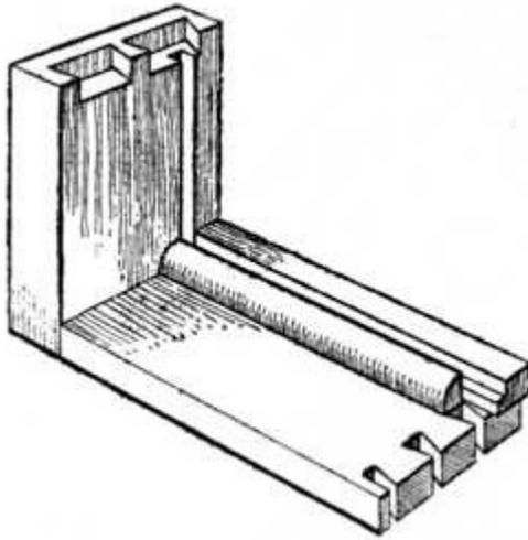
**Fig. 24.—Glueing Ploughslips to Drawer.**
