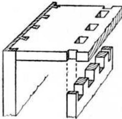
**Fig 150.—Method of Pinning.**
