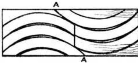
**Fig. 337.—Board Marked for Circular Jointing.**
