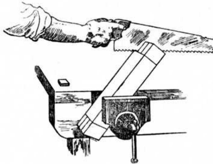
**Fig. 180.—Second Operation in Sawing Tenons.**
