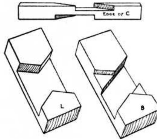
**Fig. 46.—Detail of Halved Joints in Fig. 45.**
