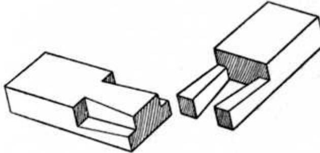
**Fig. 42.—Dovetailed Halving Joint used for Lengthening Timber.**
