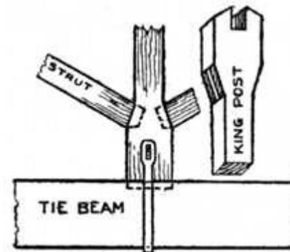
**Fig. 161.**—Roof Joints.
