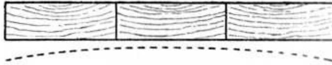
Fig. 10.—Showing Heart side of Timber one way.
