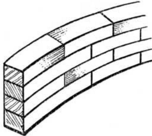
**Fig. 341.—Part of Laminated Table Frame.**
