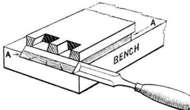
**Fig. 287.—Working a Housed and Mitred Dovetail Joint.**
