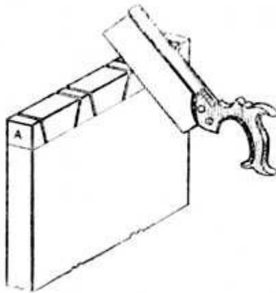
Fig. 281.—Sawing the Drawer Side.
