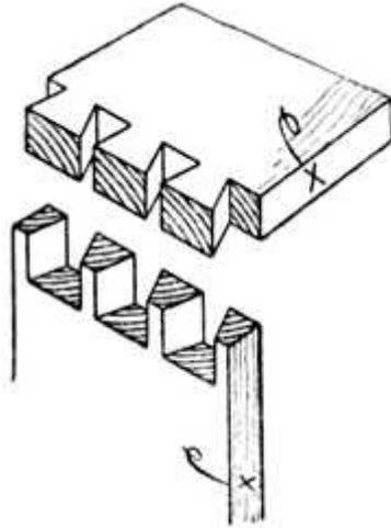
**Fig. 310.—Through Dovetailing.**
