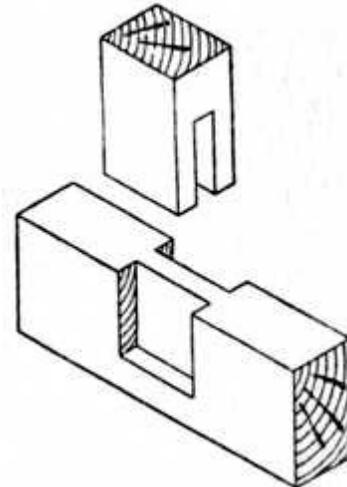
**Fig. 77.—Stopped Bridle Joint.**
