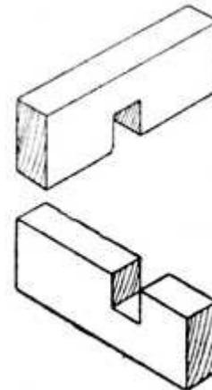
**Fig. 40.—Cross Halving Joint Edgeway**
