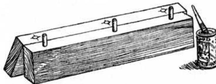
**Fig. 199.—Dowelled Joint ready for Glueing.**
