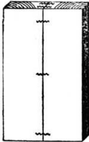
**Fig. 362.—Jointing Boards.**
