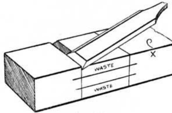
**Fig. 88.—Chiselling Operation.**
