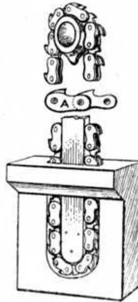
**Fig. 139.—Sprocket Wheel.**
