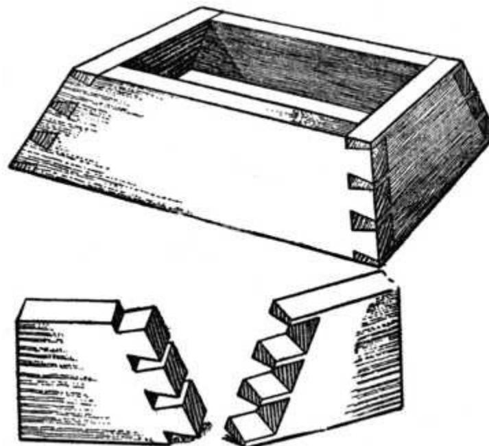
Fig. 297.—Bevelled and Dovetailed Box, showing the
