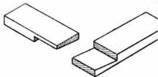
**Fig. 36.—Halved Joint with Double
