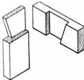
**Fig. 35.—Halved Joint with one side
