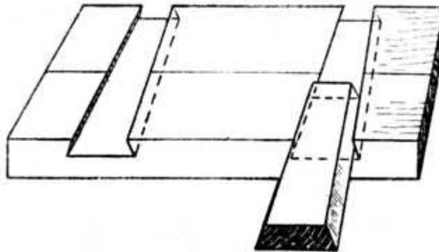
**Fig. 289.—Dovetailed Keys for Wide Surfaces.**
