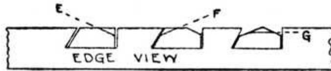
**Fig. 319.—Showing Method of Paring.**
