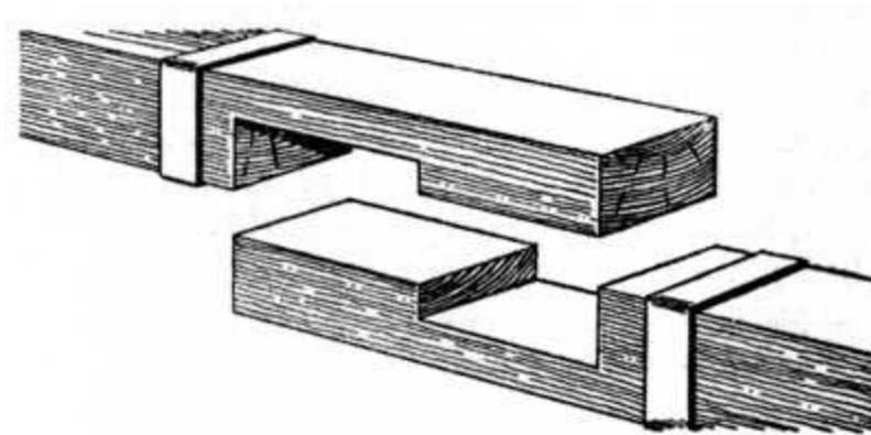
**Fig. 219.—Example of Tabled Joint with Straps.**
