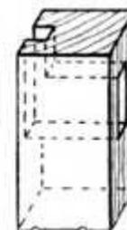
**Fig. 131.—Haunched Tenon used when Sti Grooved for Panel.**
