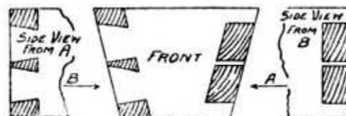
Fig. 298.—Oblique Dovetailing.
