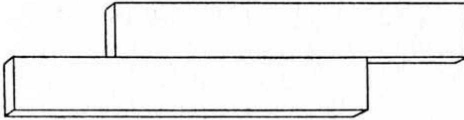
**Fig. 1.—Simplest Form of Glued or Rubbed Joint.**
