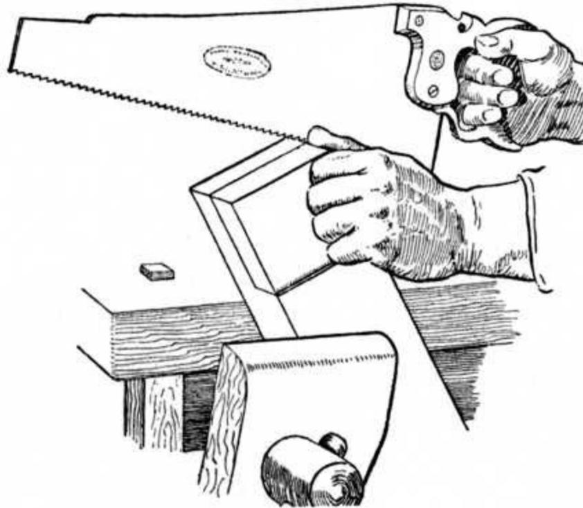
**Fig. 70.—Sawing the Cheek of a Halving Joint.**
